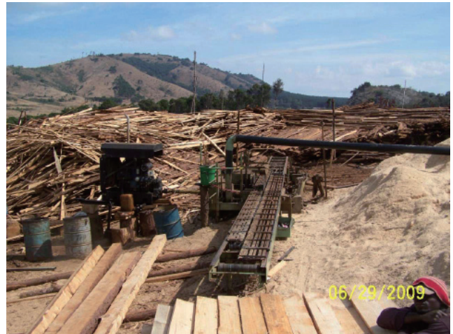
Picture 6. A KARA F2000 sawmill- one of the semi-mobile type.
