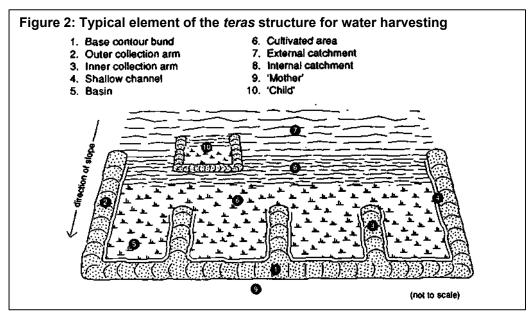
Bund height is usually 0.5m, with bases 2m wide. The dimensions vary with slope and amount of run-off expected in the area. Base bund lengths are between 50-300m (recorded maximum lengths up to 700m), with arms usually 20-100m (up to 200m). The ratios of base: arm dimensions are not fixed, but base bunds with lengths under 100m seem to have
