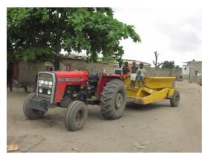
Low-technology equipment has been purchased, which will collect solid waste from sites within a *bairro* and deposit it at a site from which ELISAL will collect and transport it to the main city dump. The equipment is hauled by a tractor that can be used on narrow dirt roads. A container is left at a site inside a *bairro*, and is picked up a few days later by the tractor, which leaves another container.
