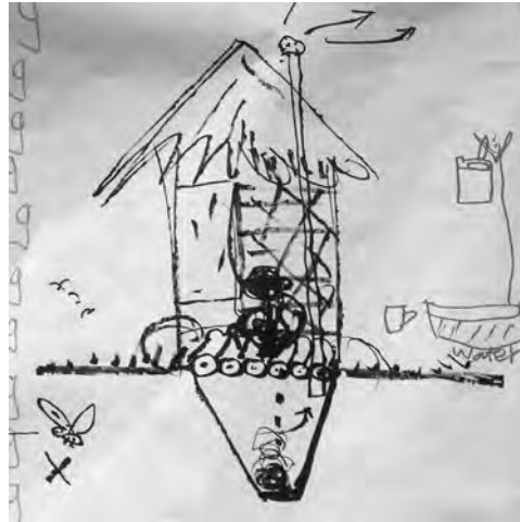
A sketch of a self ventilated improved pit latrine design, Kabengele village, Zambia.
