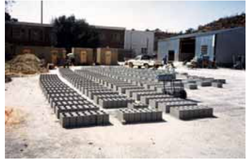
Bricks in which riversand has replaced by tailings.
