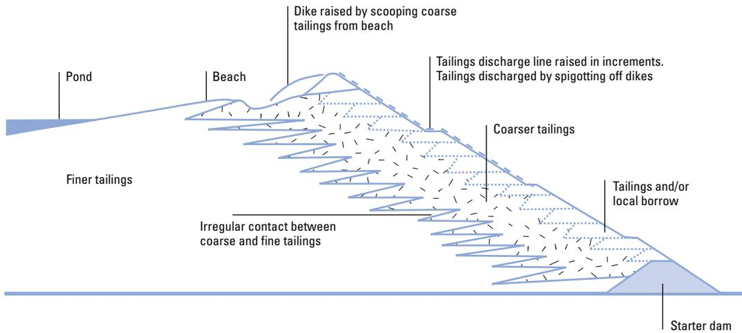
**Downstream Method of Tailings Dam Construction**
